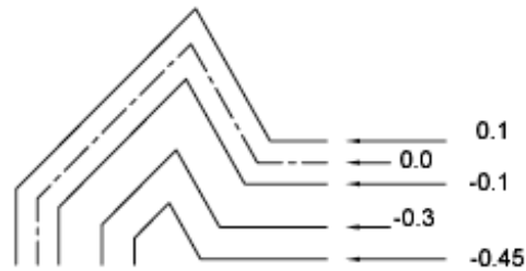
a four-element multiline, each element offset from 0.0
